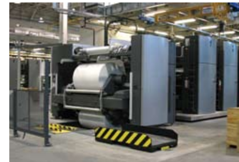
Valpak’s Goss Sunday 4000 webs print continuously in short-run batches of 10,000.
